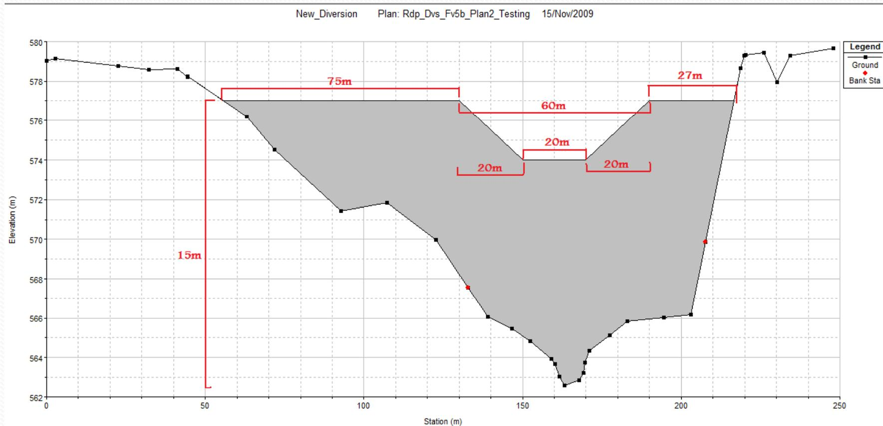
**Proposed (INLINE) Weir at Rivière du Poste downstream of the siphon**
