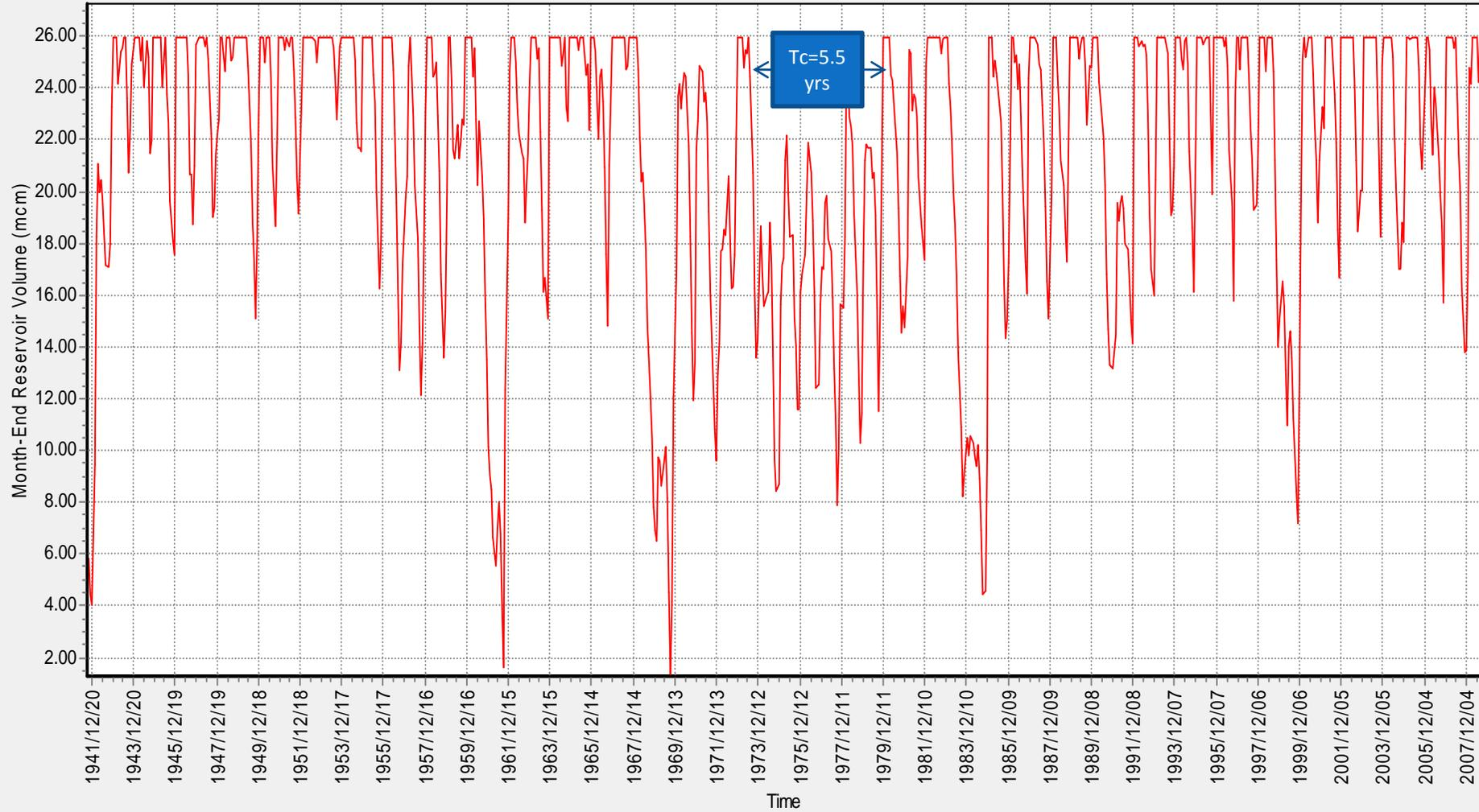
Augmented MAV Reservoir Level (when TD = 43.8Mm<sup>3</sup>/a)
