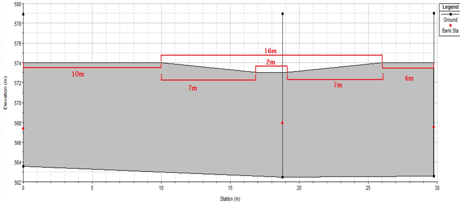
Proposed (LATERAL) Weir at Rivière du Poste downstream of the siphon
