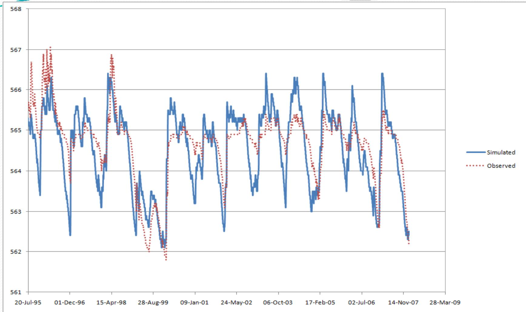
**Simulated vs. Observed Water Levels at the MAV (1995-2008)**
